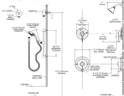
NOTE: This valve is not intended to be used as a shut-off valve. To prevent the potential of cross flow, check valves must be integral to the supply valve or installed in both hot and cold water supply lines.
